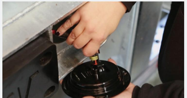
**While today's LED lamps are often designed to use dielectric grease and modular connection designs to resist moisture at the connection point, they still must be inspected regularly and the grease replaced when needed.**
