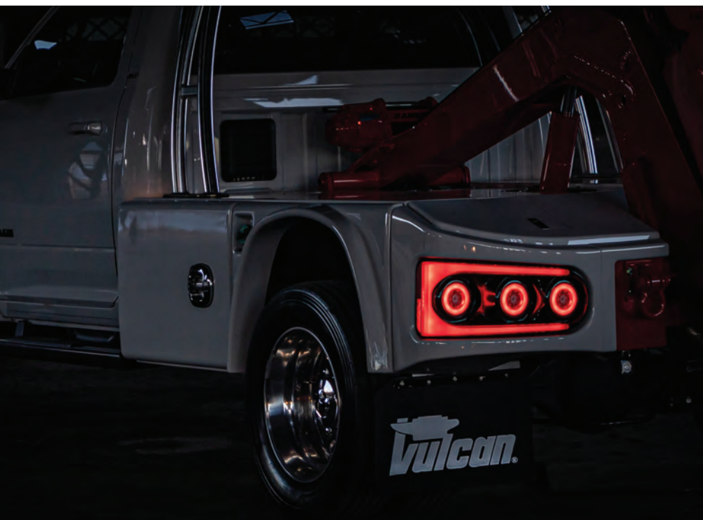
Optronics designed a tail lamp with a modular look consisting of several lamps within one modular unit housing three, 4-inch round Optronics Fusion GloLight lamps.
