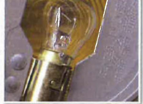
*Vibration is the most common cause of broken lamp filaments, according to Grote.*
