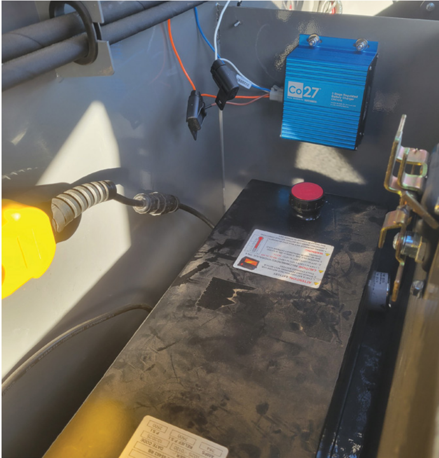
When the Co27 activates, it measures electrical resistance across the entire circuit between itself and the towing vehicle's battery, and if it detects high resistance, reduces current draw to as low as 3.5 amps to protect upstream wiring and fuses.
