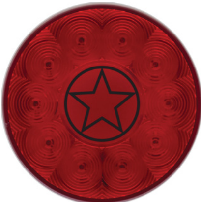
STL104 Series features 29 SMD LEDs, with 10 paired with optics and 19 further illuminating the logo portion of the light during stop and turn functions.
