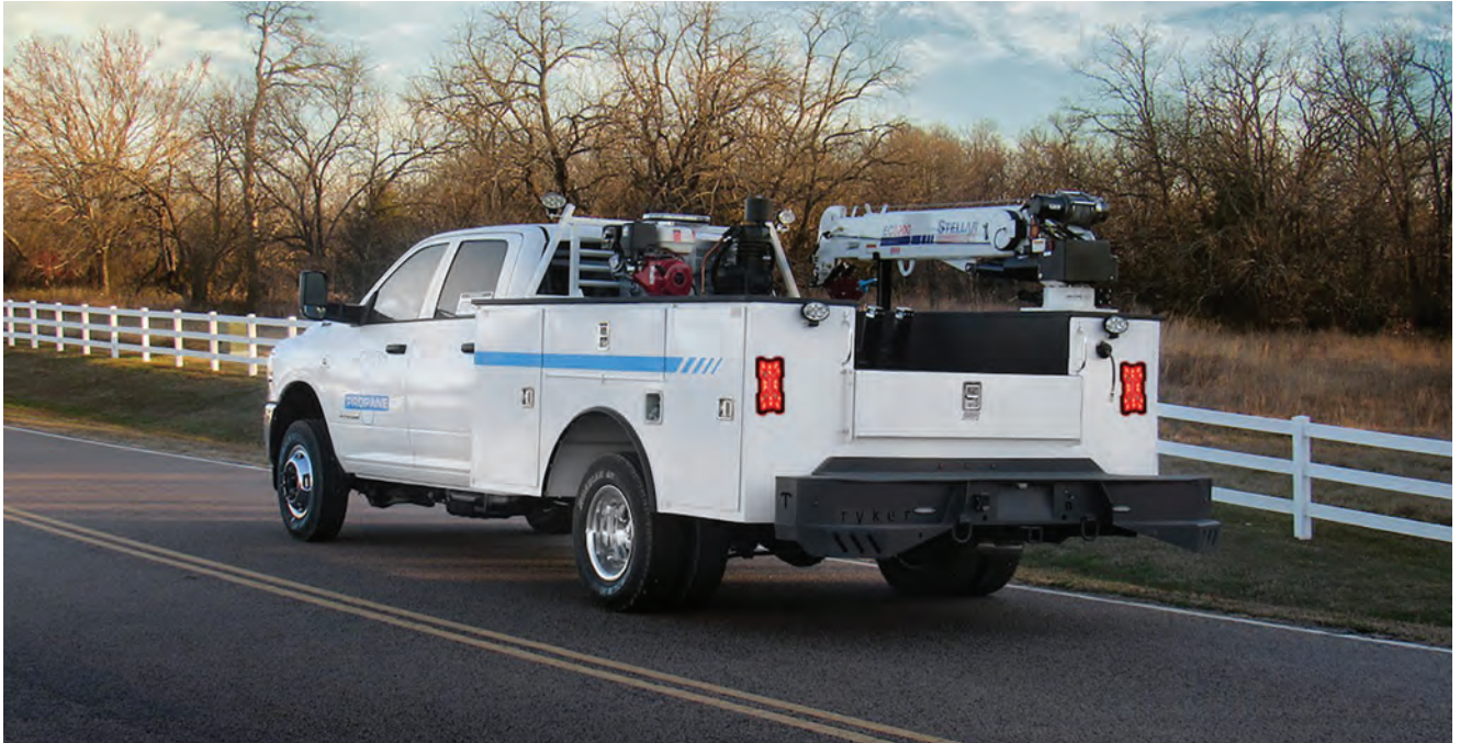
FusionX tail lights are DOT compliant, which allows the stop, turn, tail light functions to override the warning light function.
